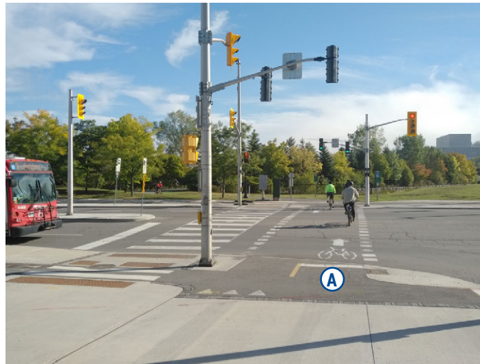
Image 5.6. Example of bicycle queueing area at Ottawa River Pathway and Booth Street
