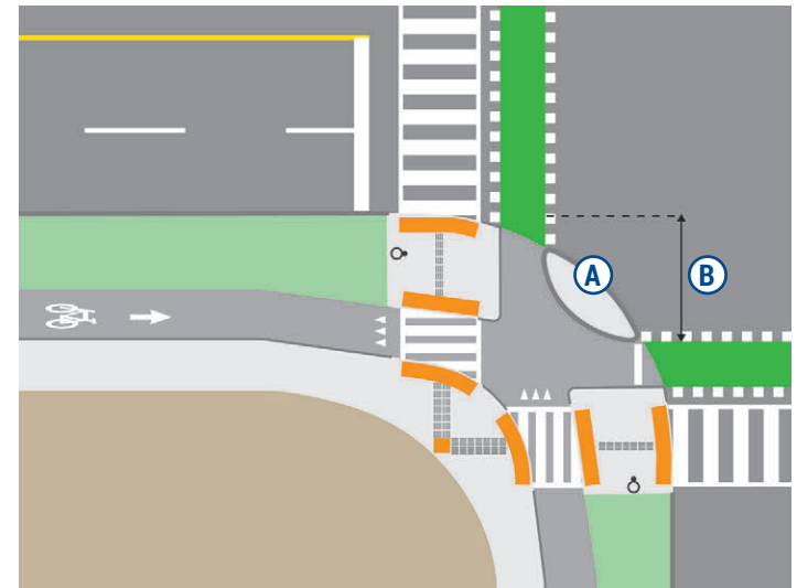
Figure 5.4. Standard protected corner with 10.0 m radius showing 5.0 m crossside setback
